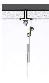
Side view of assembled mounting hardware and panel attachment
